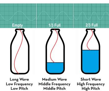
Soundwaves are measured by their **frequency**, or how many waves pass through one place in a certain amount of time. Shorter waves have a higher frequency and longer waves have a lower frequency. We hear the frequency as sounds that are higher or lower, which we call **pitch**.
